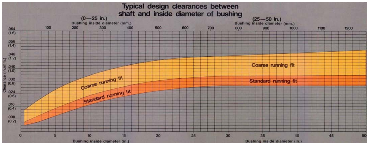
Typical design clearances between shaft and inside diameter of bushing(0-25 in.)
