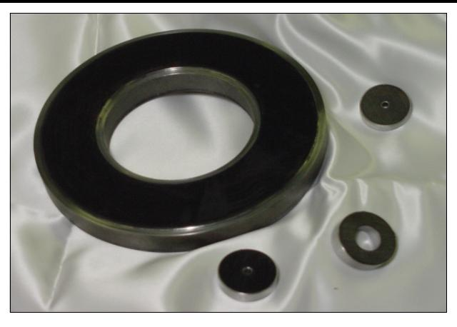
COMPACTING TOOL BEARINGS FOR SINTERED POWDER METAL PARTS. SELF LUBRICATION WITH NO NEED FOR SUPPLEMENTAL LUBRICATION SUCH AS OILS OR GREASES FOR THE LIFE OF THE BEARING. CAPABLE OF SUPPORTING DYNAMIC PRESSURES UP TO 35,000 PSI WITH VERY LOW WEAR. WILL SUSTAIN PERFORMANCE IN A TOLERABLE CONTAMINATED HOSTILE POWDER ENVIRONMENT. IDEAL FOR USE IN SUPPORT OF COMPACTING TOOLING FOR HELICAL GEARS.
